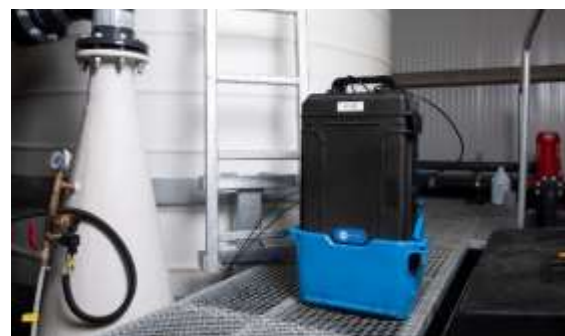
Aquamonitrix® real-time nitrite and nitrate analyser
